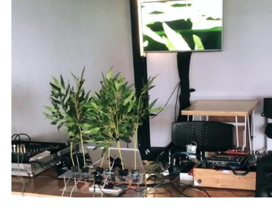
This installation consists of multiple servos embedded with artificial plants which can move so they will rub against each others. The sound from the frictions are amplified then processed through some digital effects. The movement of the plants are also live-recorded with a camera and then processed through software and visualized through the screen.
