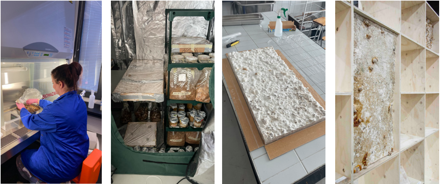
Fig. 10 The story of the panel that made me let go of control from a jar of shared reishi spawn in a glass jar donated by a neighbour, through inoculation in sterile Biofilia laboratory and first growth in grow bags to spreading into a formwork, growing again in the warm and humid tent to finally drying in room temperature over my summer vacation growing fruiting bodies and creating a fascinating surface of textures and colours. Photos by Elina Koivisto. [more photos in exposition]
