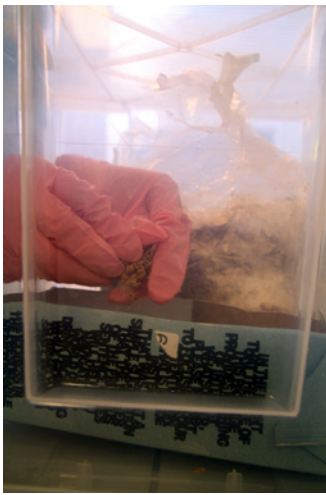
Fig. 18: A student breaking mycelium grown into wood chips into a formwork made with milk cartons. Photo by Elina Koivisto.
