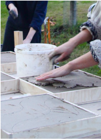
Fig. 24: Elements with clay and natural fibres being made by workshop participants on 17.9.2024. Photo by Elina Koivisto.
