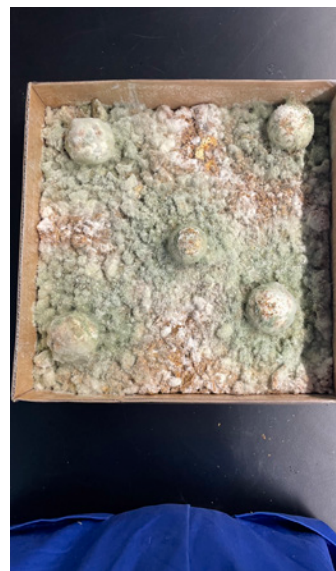
Fig. 14: Blue moulds joined the creative community uninvited preventing oyster mushroom from growing and creating a panel intended for Kudos physical structure. Photo by Elina Koivisto.
