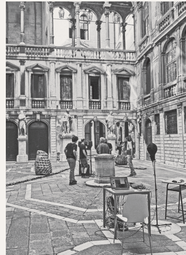
3D impulse response recording outdoors (courtyard of the Conservatorio di Musica Benedetto Marcello Venezia)
