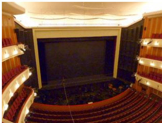
Figure 6: At the top of the picture, the concave sails of the opera in Düsseldorf can be recognized. These facilitate the communication among the musicians by reflecting sound back to the pit.
