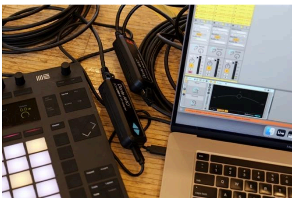
Figure 5a. USB Type-C I/O Audinate AVIO 2×2 and AVIO Analog Output Adapter 0x2 for routing. (Photo: Wilde, CC BY 4.0 DEED).
