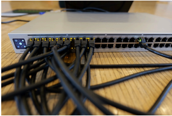
Figure 4c. LO audio over ethernet (AoE) network used during LO classes. USW-48-POE 48 port Managed Gigabit L2 L3 Switch - 48x with Gigabit Ethernet Ports with 32 POE+, students learning about computer technology networks. (Photo: Wilde, CC BY 4.0 DEED).
