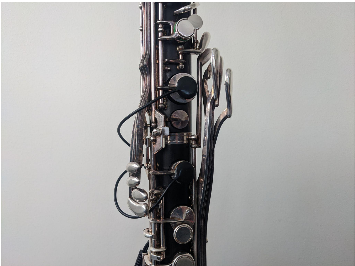
Image 7: Contact microphones attached to the pads. Photo by Jaakko Arola.
