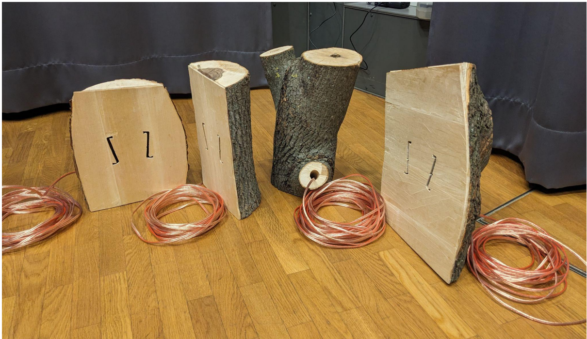
Image 9: Wooden bark loudspeakers. Photo by Jaakko Arola. Three loudspeakers with a transducer attached to a soundboard and one branch section loudspeaker with a speaker element inserted inside (second to right).
