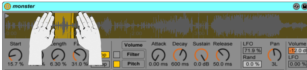
Figure 6: Sound manipulation: left hand marks the beginning of the play range and the right the determinate the end point. This range is updated in real-time.
