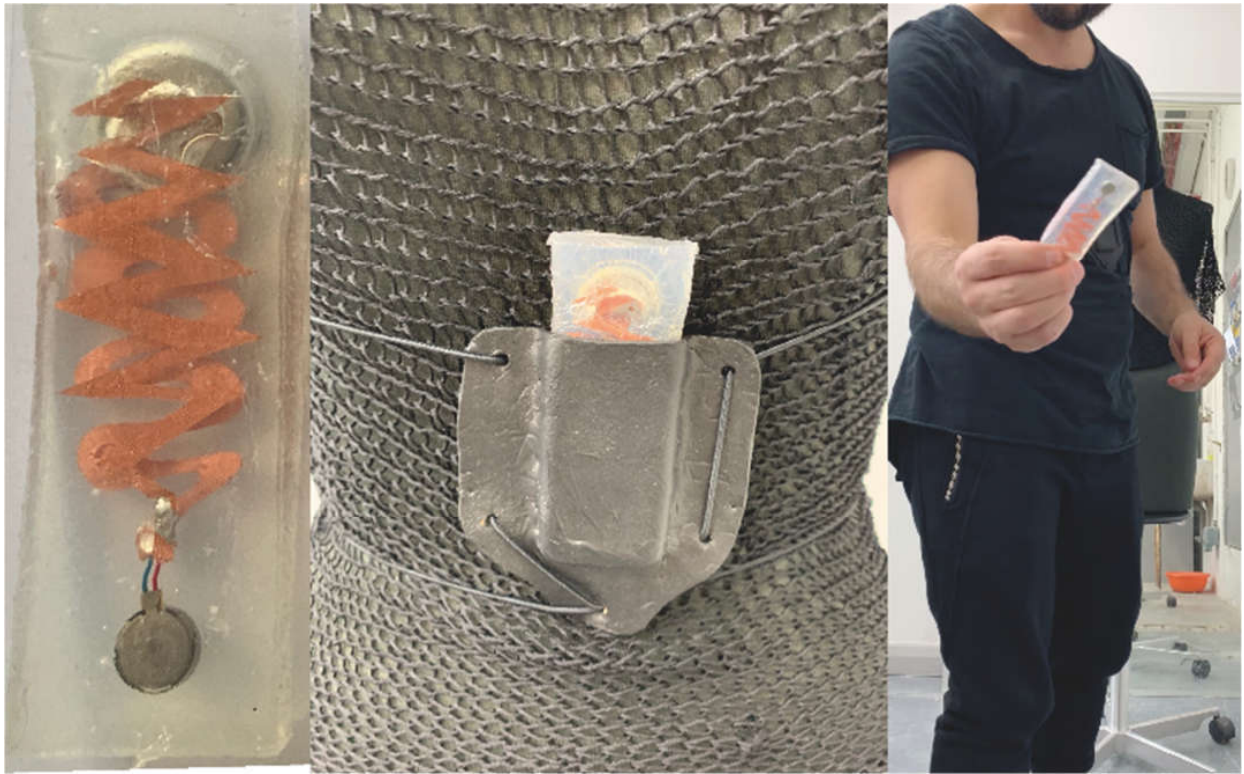
Figure 2. (2018) Pager motor suspended in silicone with e-textile as conductor; moulded leather casing on front abdomen
