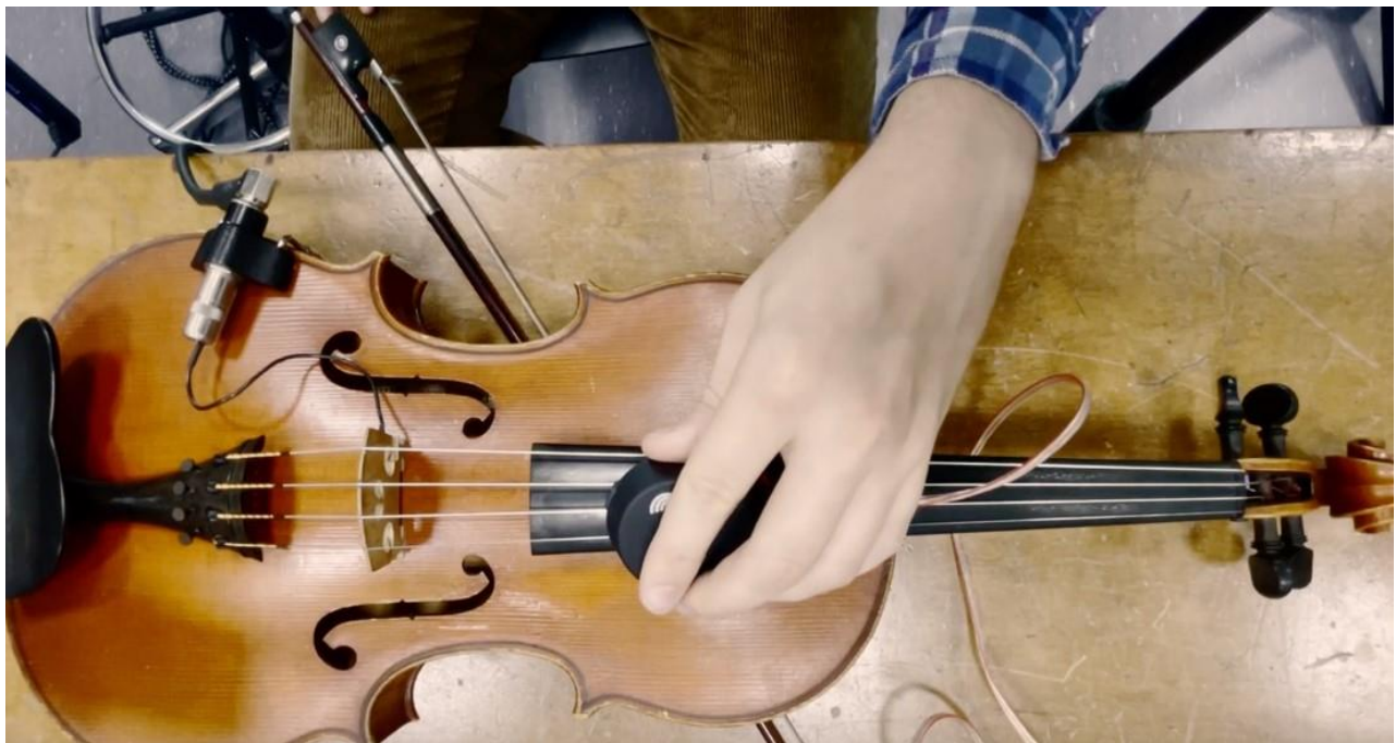
Figure 7, The transducer setup for Navigations. One transducer is placed on the bottom of the viola on the lower bout, while the second is in my hand.
