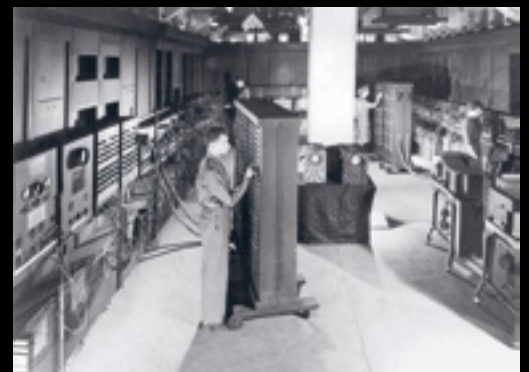
16 Corporal Irwin Goldstein sets the switches on one of the function tables of the ENIAC, the first electronic, general-purpose computer, Moore School of Electrical Engineering, Philadelphia, 1946.
