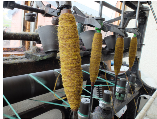
Fig. 3.1. A single-width domestic Hattersley loom, one of the two kinds of handlooms used to weave Harris Tweed today. Introduced to the islands in the early 1900s, the Hattersley loom became the most common equipment for producing Harris Tweed throughout the twentieth-century, and is still used today primarily by weavers working as ‘independent producers’. Its more recent counterpart, the double-width Bonas Griffith loom (Fig. 3.3) was introduced in the 1990s (following discussions and experiments taking place since the 1970s, see Hunter 2001:287-355), and is most commonly used today by weavers completing mill orders.
