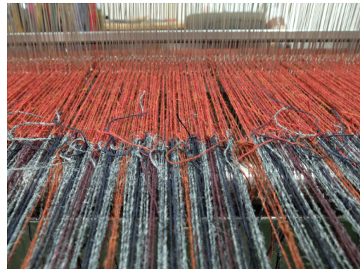
Fig. 6.2. Joana learning to 'tie-in' on a double-width Bonas Griffith loom. (Photo by G.M.)
