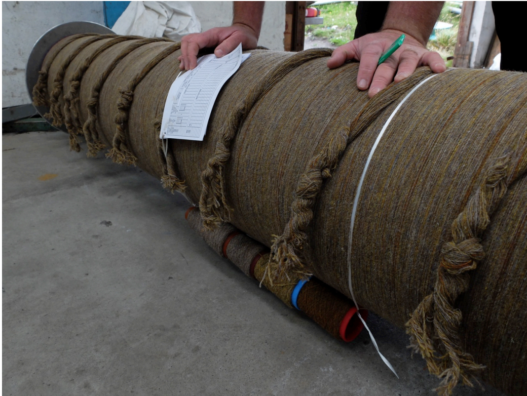
Fig. 2.1. A mill worker checks the ticket with weaving instructions on a ‘beam of five’ (that is, a warped beam with enough yarn to weave five lengths of tweed – each piece about 58m long), before placing it on the back of the tweed van for delivery.
