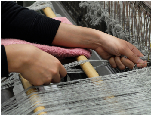
Fig. 6.2. Joana learning to 'tie-in' on a double-width Bonas Griffith loom. (Photo by G.M.)
