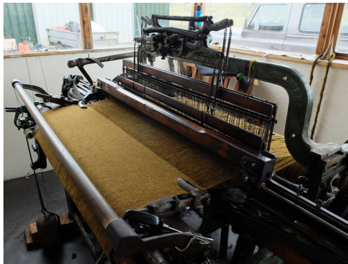
Fig. 3.1. A single-width domestic Hattersley loom, one of the two kinds of handlooms used to weave Harris Tweed today. Introduced to the islands in the early 1900s, the Hattersley loom became the most common equipment for producing Harris Tweed throughout the twentieth-century, and is still used today primarily by weavers working as ‘independent producers’. Its more recent counterpart, the double-width Bonas Griffith loom (Fig. 3.3) was introduced in the 1990s (following discussions and experiments taking place since the 1970s, see Hunter 2001:287-355), and is most commonly used today by weavers completing mill orders.
