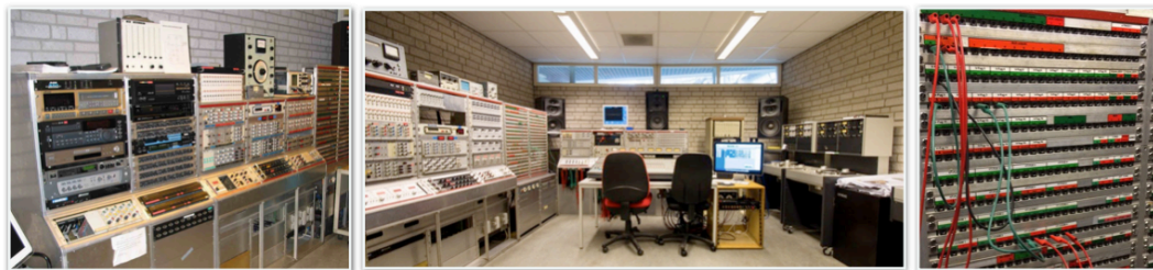
Figure 1.1. Analogue studio Bea-5 with the patch-panel (on the right) where all ins and outs are located.
