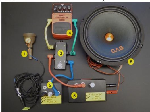
Figure 1. Module based Thranophone (MBT) with Bronze/PLA mouthpiece.
