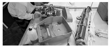
First step is to unmount the machine and disassemble all the plastic covers that are possible to remove. Other than hands we also needed screwdriver.
