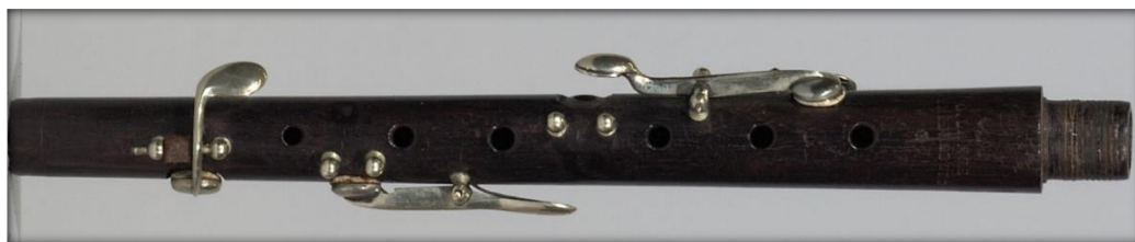
Figure 633: C. Lange C Piccolo, St. Petersburg, a1878-p1882, (Part only), Cocuswood(?), stained dark, nickel silver keys, 20.4 cm, Key Holes System: 6 keys, post, and rod, direct mount. 2335
