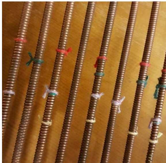
Figure 3.5. Marking of the harmonic positions on the piano string. From low to high, respectively: 11th harmonic (yellow), 7th harmonic (white), 10th harmonic (green), and 13th harmonic (red).
