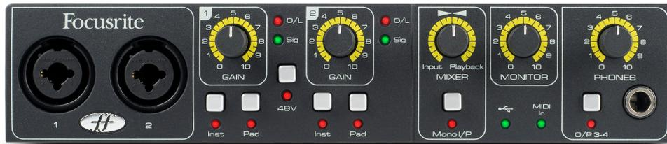
An audio interface is a device that converts an analog audio signal into digital signal. The audio interfaces can be connected to a computer through USB, Firewire or Thunderbolt plugs.
