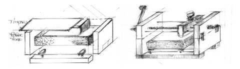
The height of the roller is adjustable, depending on the thickness of the stone, and for a more functional solution, its base can also be adjusted for stones of different thicknesses.
