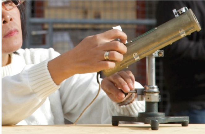
Figure 64, A Pyrheliometer is an instrument that reveals the difference between the energy level in a tube like cavity when the sun shines directly into it and when it is closed.
