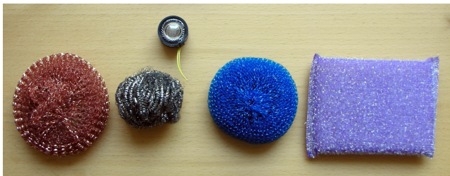
Figure 2: Different synthetic materials (sponges and steel wool) that work well together with dynamic microphone elements (seen at the top).
