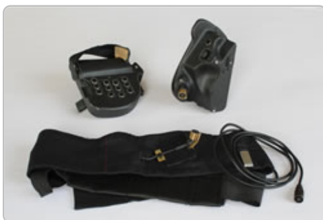
Figure 4. The "backup" version of the controller pair of the Strophonion together with the hip belt and cable for the ultrasonic distance sensor. Image © Janina Janke, 2014. [Click image to enlarge] ( http://econtact.ca/18_3/images/nowitz_strophonionV2-JJ.jpg )
