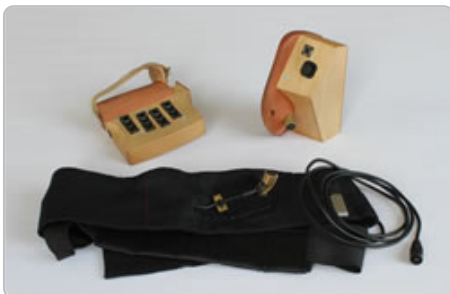
Figure 1. The Strophonion's controller system, consisting of the right-hand controller (on the left in the image), the left-hand controller (right) and the hip belt. Image © Janina Janke, 2014. [Click image to enlarge] ( http://econtact.ca/18_3/images/nowitz_strophonion-JJ.jpg )
