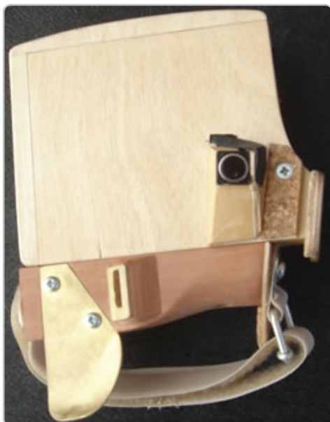
Figure 8. The shift (or modifier) key and the pressure sensor on the right-hand controller are both operated by the thumb. Image © Alex Nowitz, 2011. [Click image to enlarge] ( http://econtact.ca/18_3/images/nowitz_strophonion-altmode.jpg )
