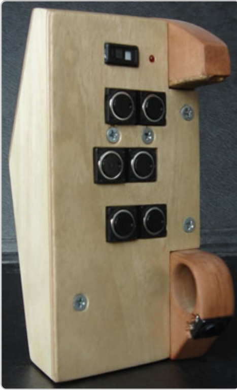
Figure 10. Front of the left-hand controller showing the cork-lined support for the index finger (top right), the six buttons, the little finger holder and “panic” button (bottom right). Image © Alex Nowitz, 2011. [Click image to enlarge] ( http://econtact.ca/18_3/images/nowitz_strophonion-LHfront.jpg )
